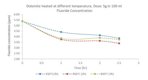
It wasobserved that dolomite calcined at 850°C shows higher fluoride removal. Various studies also show that, at 650°C, only magnesium ions get active; whereas at 850°C, calcium also gets active. By the above graph, we can conclude that fluoride removal is best when activated at 850C (2h), as both calcium and magnesium are active and would make complexes with fluoride result in better removal.
